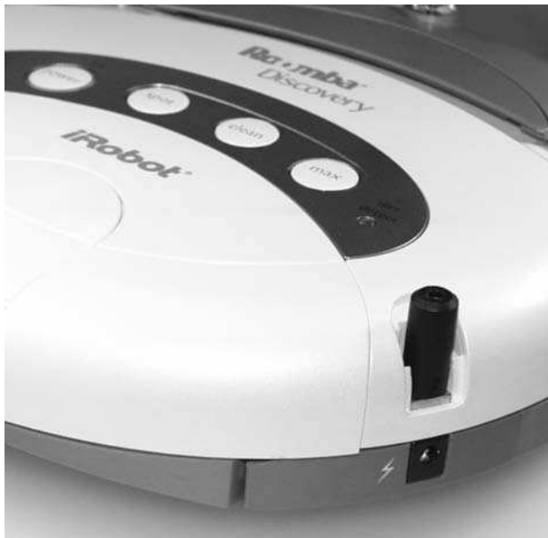
FIGURE 16-1: Roomba Mind Control microcontroller code stick plugged into the Roomba Discovery model
