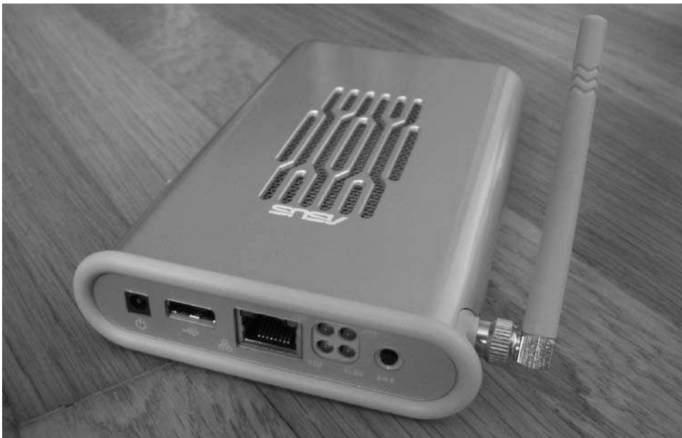
FIGURE 14-2: Asus WL-HDD, about as big as a 3.5" hard drive
