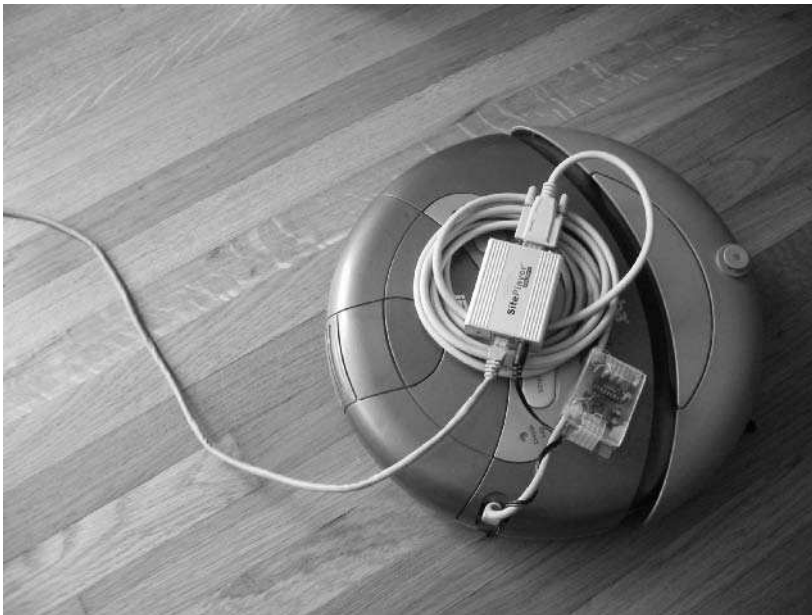
FIGURE 11-12: SitePlayer Telnet System hooked up to Roomba by way of serial tether
