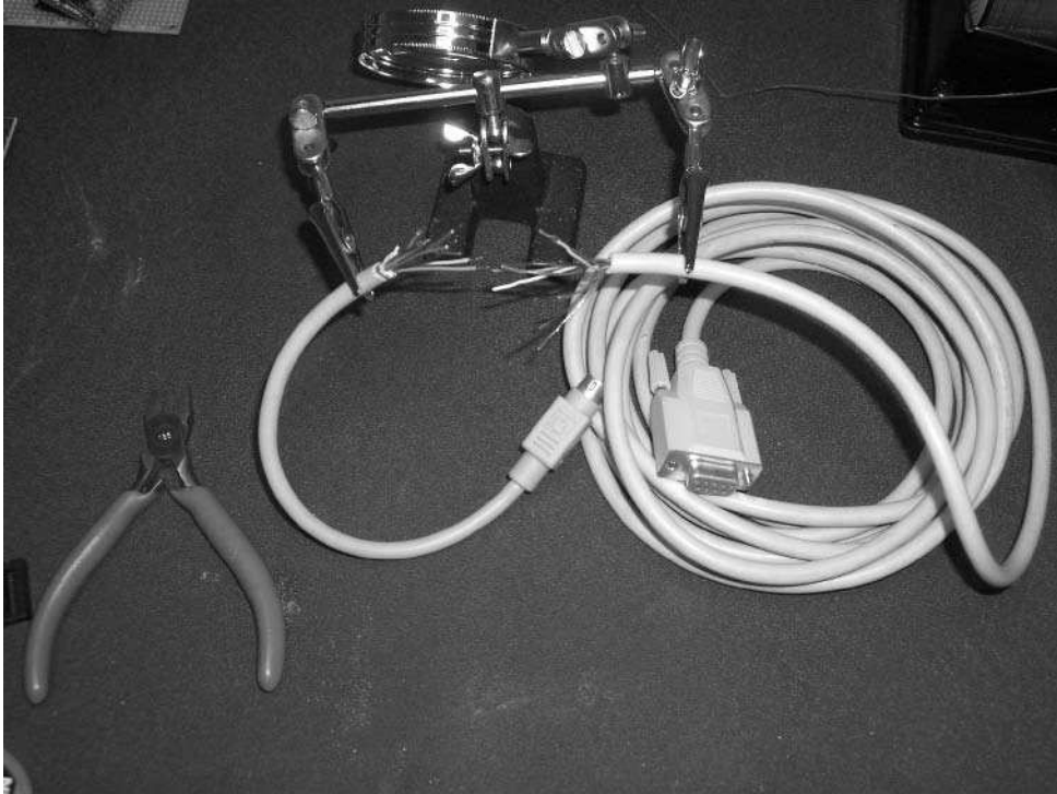
FIGURE 3-8: Mini DIN 8 and DB-9 cables in the third-hand tool, stripped and tinned for the circuit
