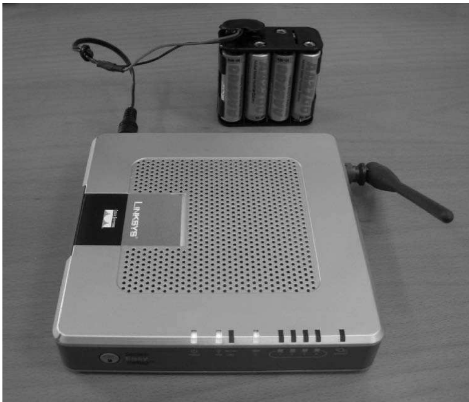
FIGURE 15-6: Power cable and battery pack in use
