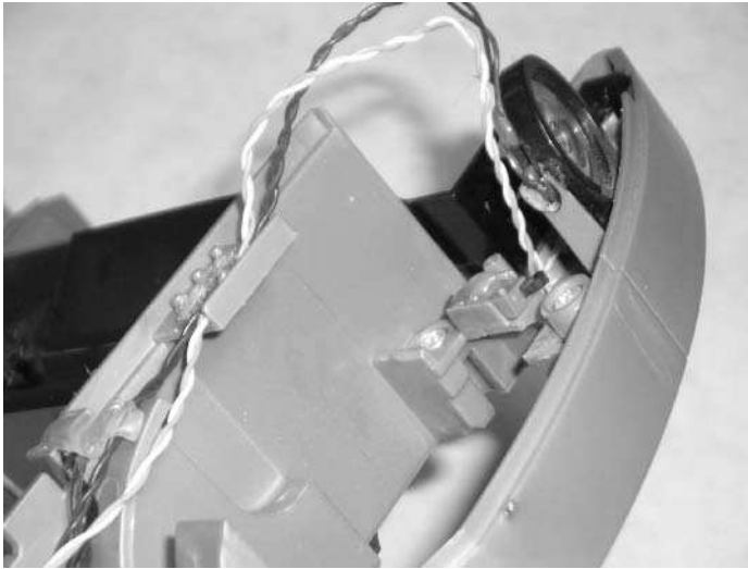
FIGURE 6-6: Wheeldrop sensor, a microswitch
