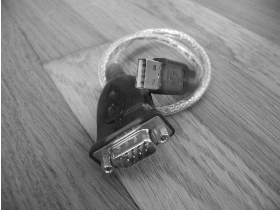
FIGURE 14-9: Generic USB-to-serial adapter, uses PL2303 chip
