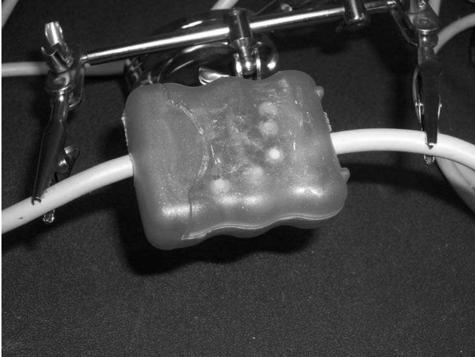
FIGURE 3-13: The circuit in a nifty blue enclosure made from a dental floss container
