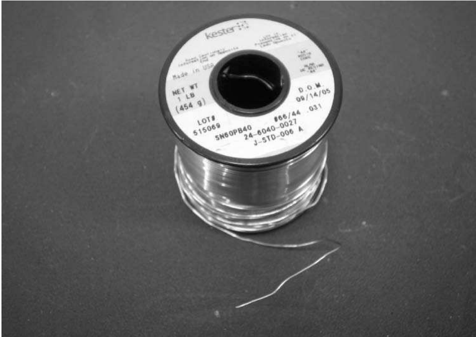
FIGURE A-2: Lead solder, 60/40 .031" rosin flux core
