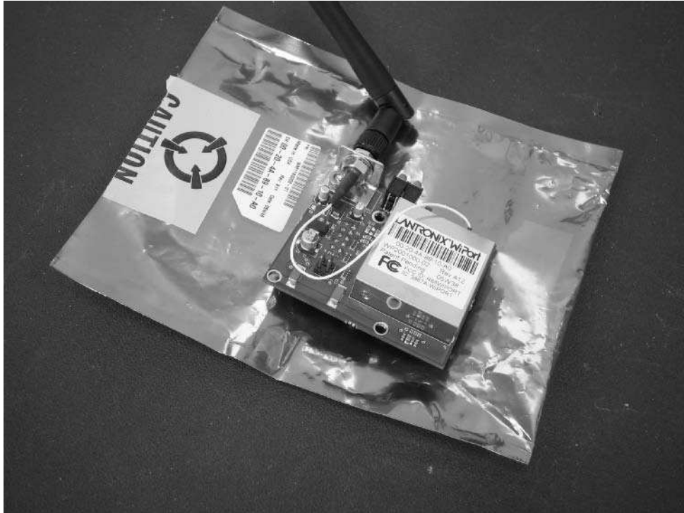
FIGURE A-22: Anti-static bag with sensitive component on top
