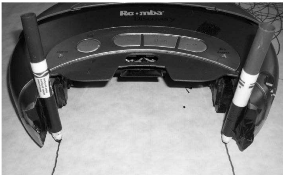
FIGURE 9-3: Duct-taped markers in the dirt bin area of Roomba
