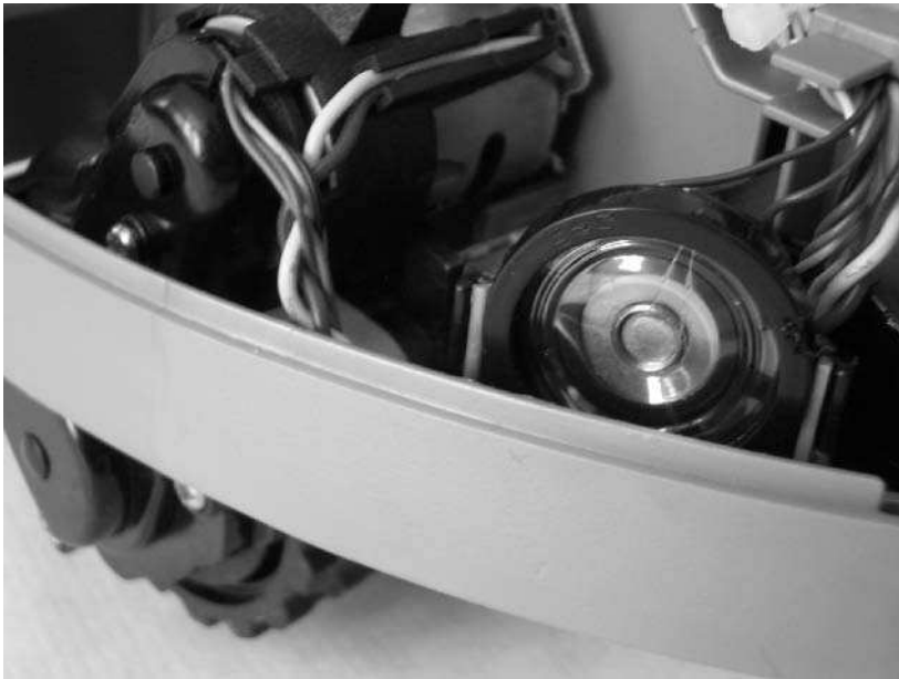
FIGURE 8-2: Piezo beeper inside Roomba
