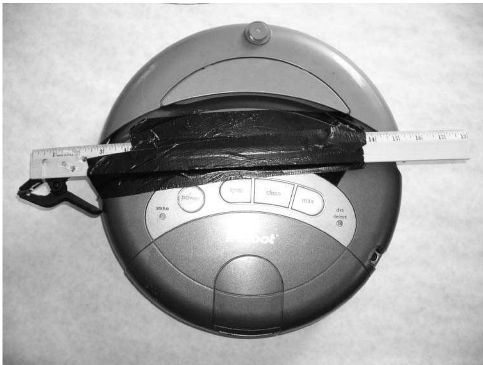
FIGURE 9-6: Ruler and clamp attached to Roomba
