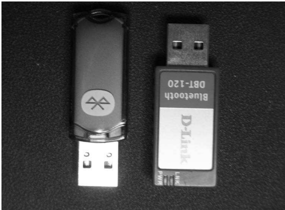
FIGURE 4-2: USB Bluetooth dongles for computers without Bluetooth
