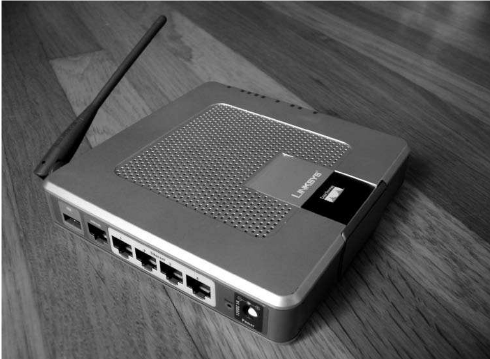
FIGURE 15-1: Linksys WRTSL54GS; note the USB port
