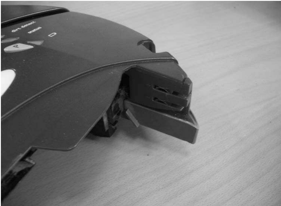
FIGURE 16-13: Vacuum motor connector, a powered output port
