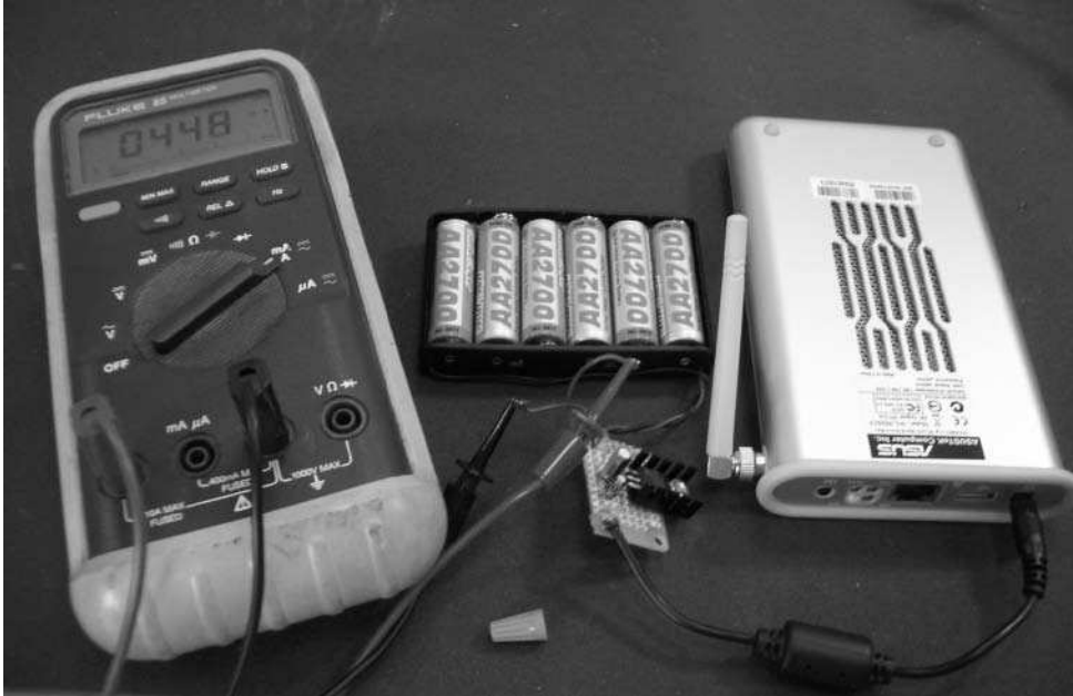
FIGURE 14-13: Testing current draw of the WL-HDD
