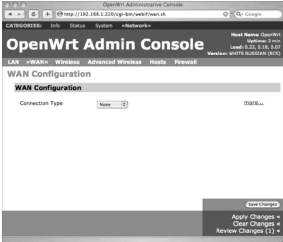
FIGURE 14-7: Disabling the WAN port in OpenWrt
