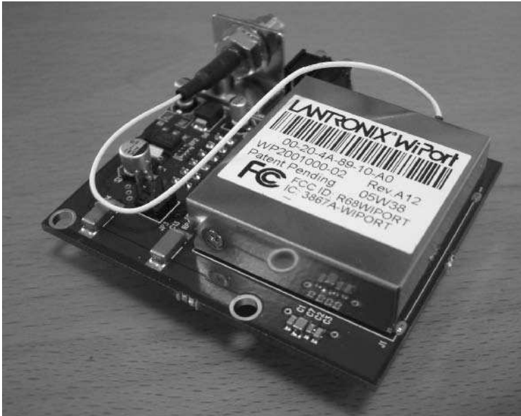
FIGURE 12-2: Lantronix WiMicro board, with WiPort attached
