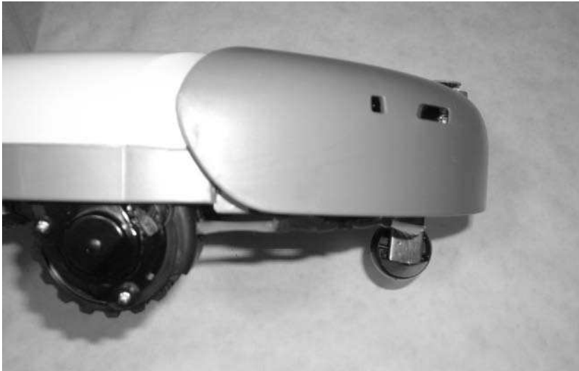
FIGURE 6-5: Wall sensors, an optical object detector
