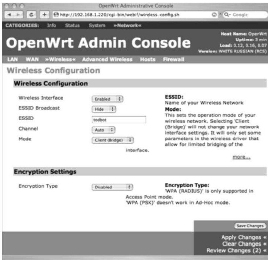
FIGURE 14-8: Configuring OpenWrt as a wireless client
