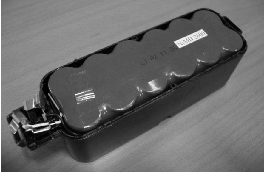
FIGURE 16-14: Battery pack partially apart
