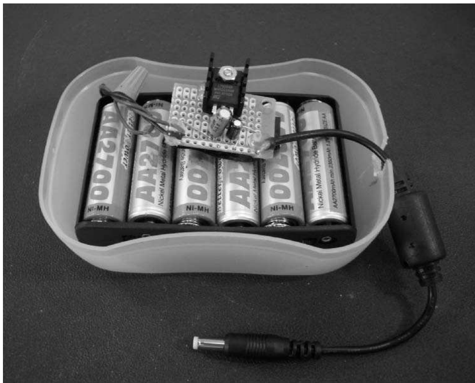
FIGURE 14-12: The power supply constructed and in its enclosure
