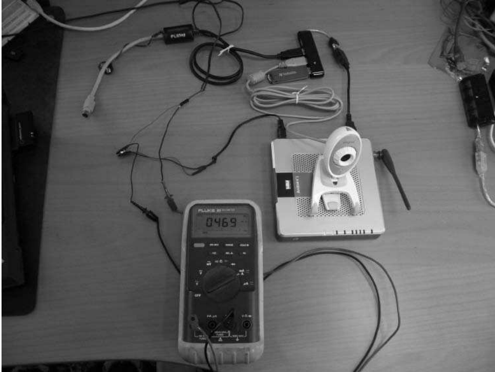
FIGURE 15-19: Measuring current of the webcam taking pictures to flash drive, with Internet access
