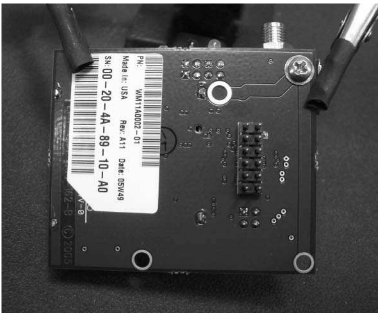
FIGURE 12-3: Underside of WiMicro with hacker-friendly 0.1" header pins
