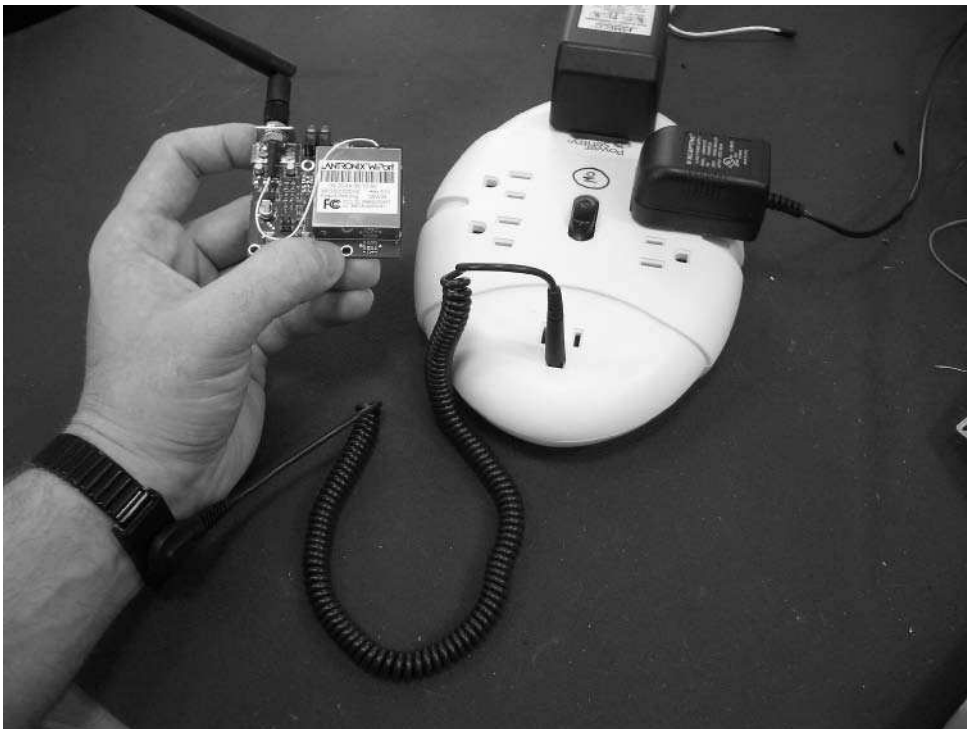
FIGURE A-21: Grounding strap for yourself, plugged into ground socket
